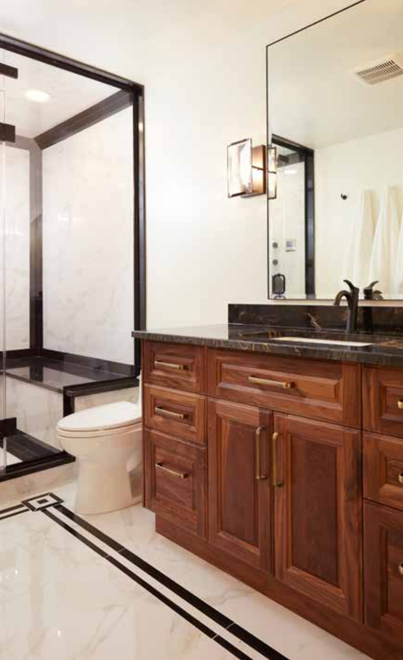
A walnut vanity houses a Magma granite countertop in the downstairs bath where porcelain floors in a marble aesthetic display Absolute Black granite inlays. The generous steam shower shares consistent black granite details and porcelain wall tile.
